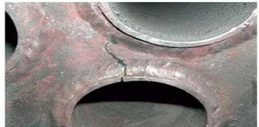
Stress cracking in the tube plate of a firetube boiler.
