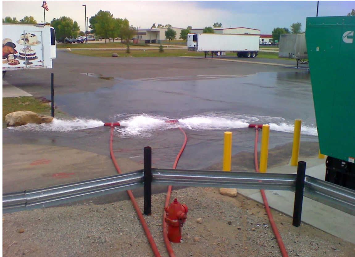
Fire Pump Test
